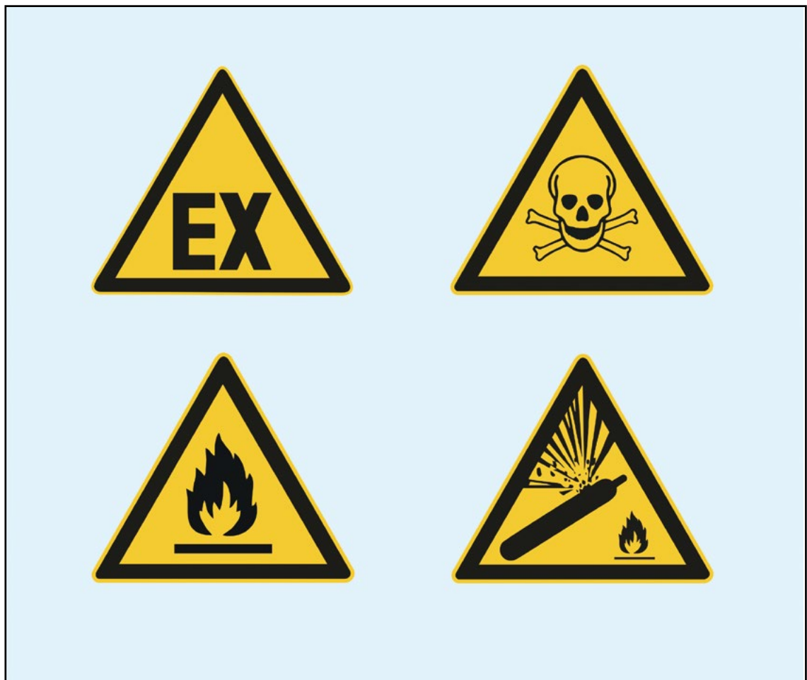
Figure 13: Main hazards associated with the storage and use of LPG: Explosion, fire and poisoning hazards, exploding gas cylinders
