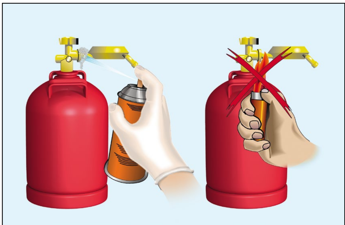
Figure 40: Leak test on LPG systems
