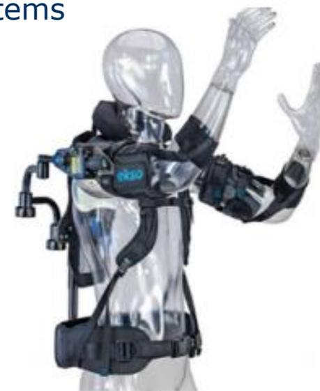
**Commercially available upper-limb passive exoskeleton**
