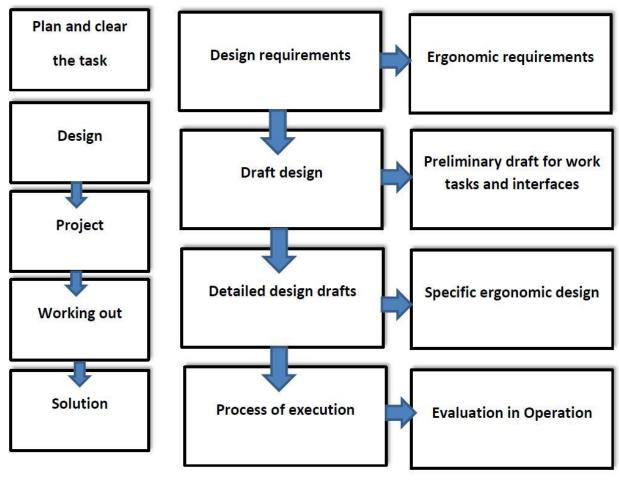
Process of planing According to EN 614-1:2009-09 under rquest to ergonomic principles
