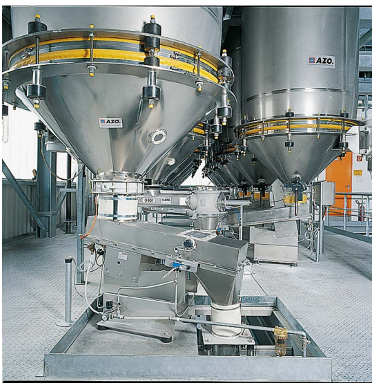
Figure 26: Silo emptying via a vibrating chute (left: AZO GmbH + Co. KG)
