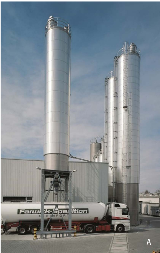
Figure 24: A): Silo emptying via a loading telescope (AZO GmbH + Co. KG)
