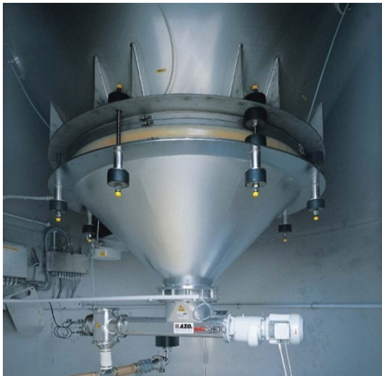
Figure 25: Screw feeder (left: AZO GmbH + Co. KG)
