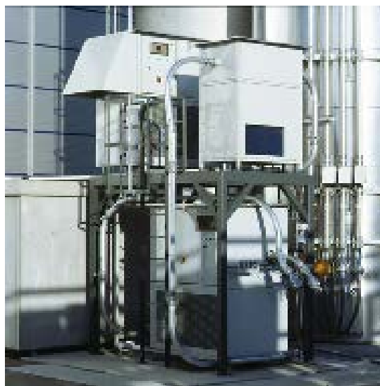
Figure 14: Stationary blower with integrated spark barrier and downstream cooler for conditioning the conveying air. (AZO GmbH + Co. KG)
