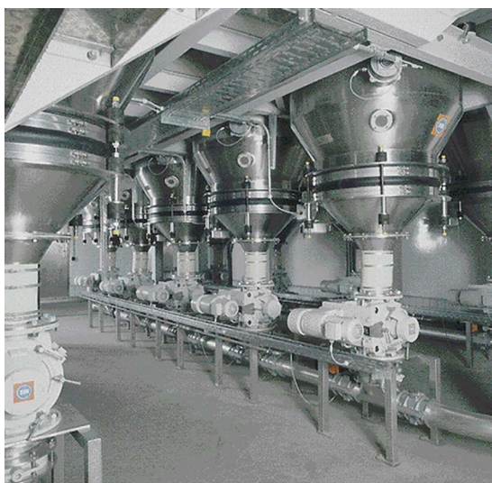
Figure 31: Silo row with discharge into pneumatic conveying lines by means of rotary air lock (AZO GmbH + Co. KG)
