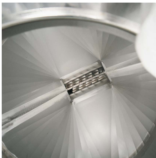
Figure 34: Silo cone with horizontal clearing screw (right: AZO GmbH + Co. KG)
