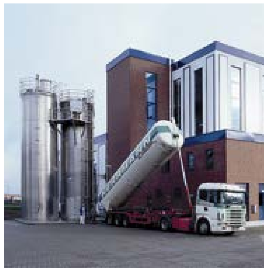
Figure 13: Silo vehicle in tipping position for filling the storage silos. (AZO GmbH + Co. KG)
