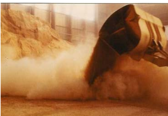
Figure 19: Dust cloud formation during open bulk handling (Prof. Siegfried Radandt)
