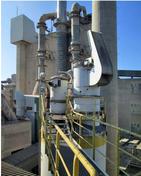
Figure 4: Separator with pressure venting flap on buffer tank (AZO GmbH + Co. KG)
