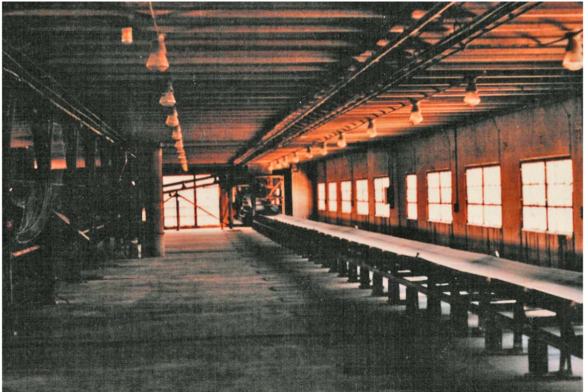
Figure 40: Silo floor with conveyor belt and splinter-free window elements as pressure venting (Prof. Siegfried Radandt)
