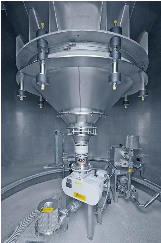
Figure 32: Silo discharge with vibrating floor and rotary air lock (AZO GmbH + Co. KG)
