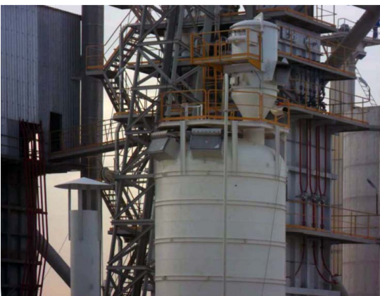
Figure 5: Silo filling via cyclone separator with lateral explosion venting (AZO GmbH + Co. KG)
