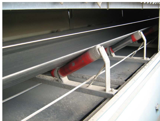
Figure 28: Belt conveyor for transporting large quantities of product over long distances (AZO GmbH + Co. KG)
