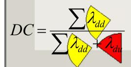
probability of detected dangerous failures probability of total dangerous failures
