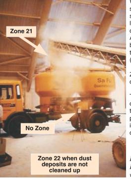
When a silo truck is filled with corn seed using an open conveyor belt as shown in Figure 6, the lower explosion limit is not exceeded except in the close vicinity of the discharge point. A zone is not allocated to the area beyond the discharge point provided that the area is cleaned each shift (elimination of dust deposits).
