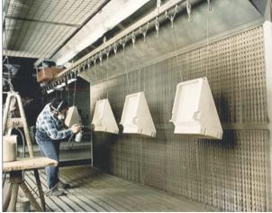
controlled by means of a flow detector in the exhaust air. The average flow rate of fresh air over the work pieces is 0.2-0.4 m/s. This provides 100-200 changes of air per hour within the paint spraying booth. Thus any explosive atmosphere which is formed is prevented from spreading and is rapidly diluted such that the formation of a hazardous explosive atmosphere can be excluded. For these reasons the inside of the booth is classified as non-hazardous i.e. no zone.
