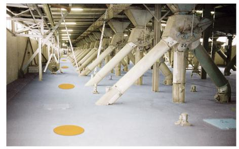
*Figure 1: Example of "good housekeeping" of the floor over a silo complex. Check marks are clearly visible, therefore non-hazardous area (no zone)* The housekeeping must be such that the check marks on the floor are always visible.
