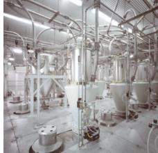
*Figure 3: Pneumatic conveying plant*
