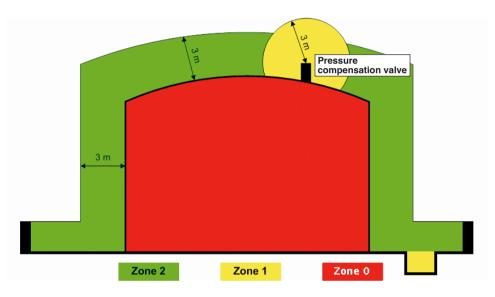
*Figure 17: Area classification drawing for an external storage tank with a fixed roof containing highly flammable liquid* [10]
