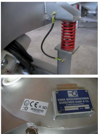
Fig. 23: Vibro screener (left). Right: Detail of earthing and tag plate which indicates that the screener is category 3D (externally).
