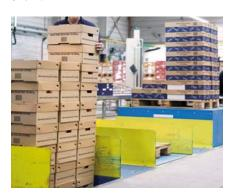
If it is not possible to use a palletizing aid that can be lowered into the floor, make sure to use a scissor lift table or trolley. This avoids deep bending when depalletizing/palletizing the lower pallet layers.
